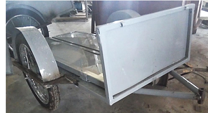
Figure 18: Un-mounted CPD motorcycle trailer (collapsed) showing the hitching point
