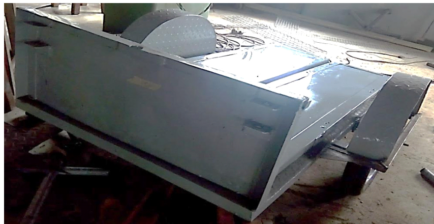
Figure 17: Un-mounted CPD bicycle trailer (collapsed) showing two hitching points
