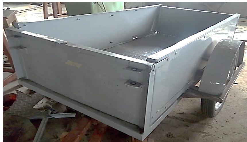
Figure 16: Un-mounted CPD bicycle trailer showing two hitching points
