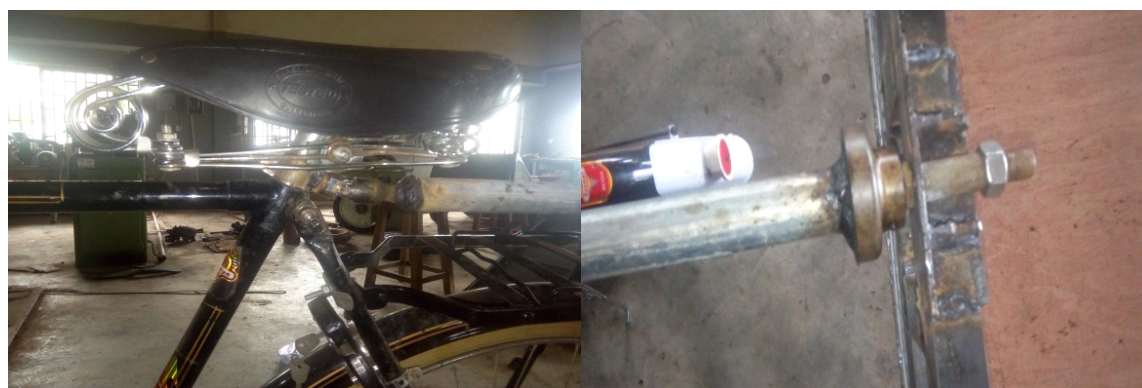
Figure 8: Hitching system for bicycle WMD trailer
