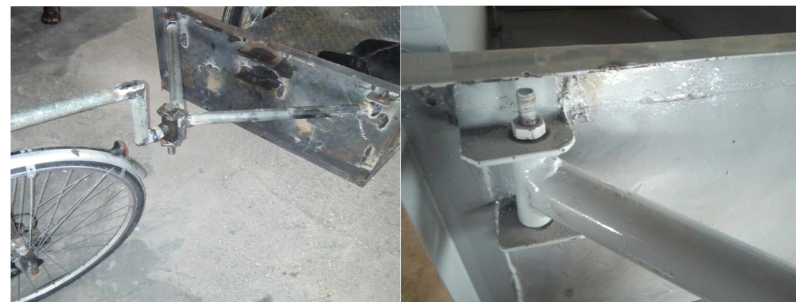
Figure 9: Hitching system for bicycle FPD and CPD trailers
