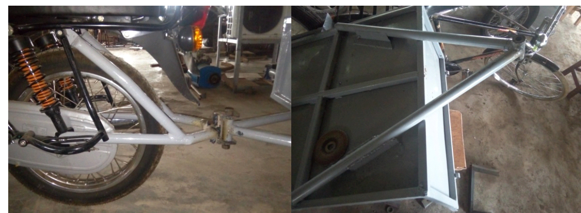
Figure 10: Hitching system for motorcycle FPD and CPD trailers
